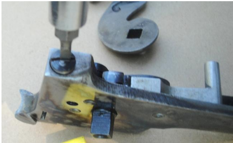
Tighten magazine screw into base of lock plate
