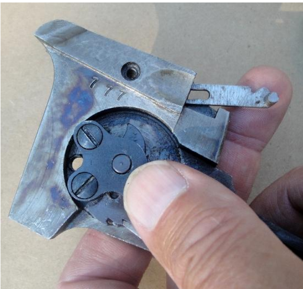
Slide pellet cut off arm into slot
