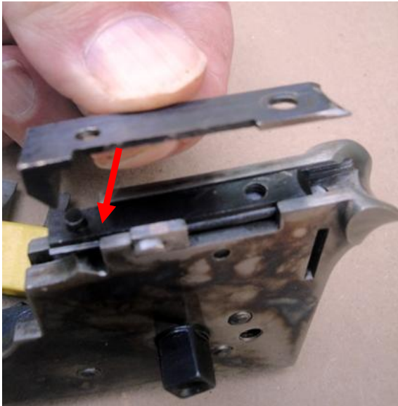
Install pellet cover spring-line up with cover nub
