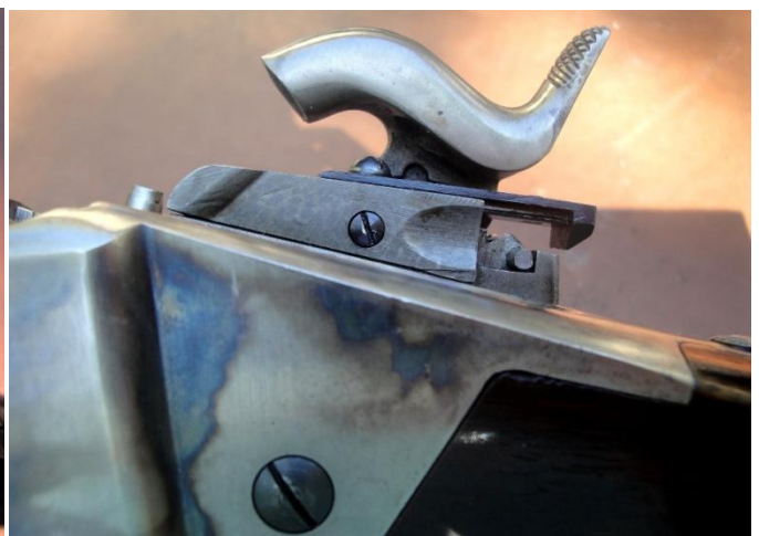
Right: side view of the Garrett Sharps lock plate showing the magazine cover/spring assembly pushed rearward for loading.
