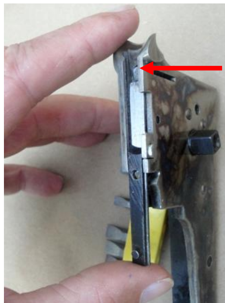
Slide pellet cover in slot (red arrow-top of plunger/magazine well)
