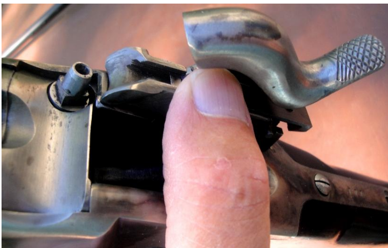
Left: sliding back the magazine cover/spring/screw.
