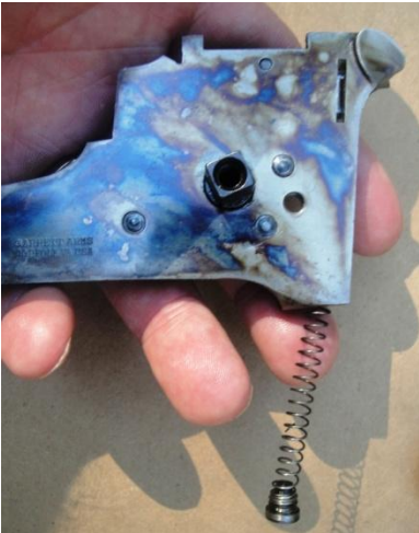
Insert plunger/spring assembly in well
