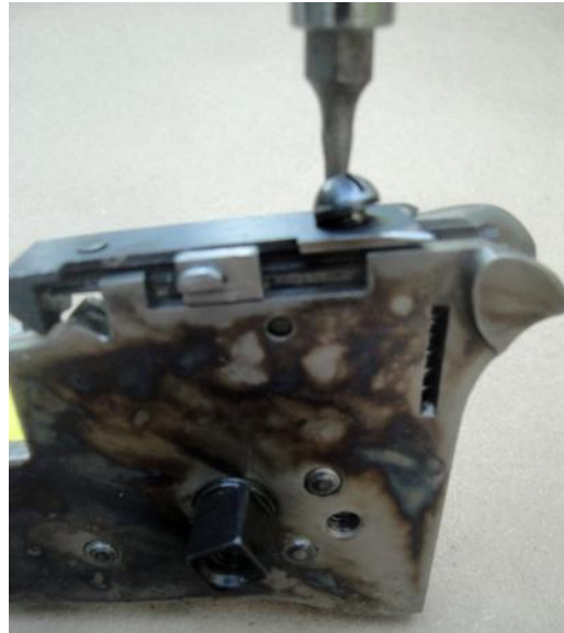
Secure spring cover screw; align feeder arm with hammer
