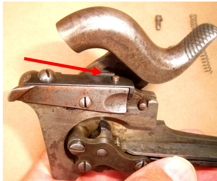
Completed pellet primer system; note mortise on inside the hammer-that mates with pellet feeder arm nub (the mortise is featured on all reproduction Sharps arms, even though they lack the pellet feeder system).
