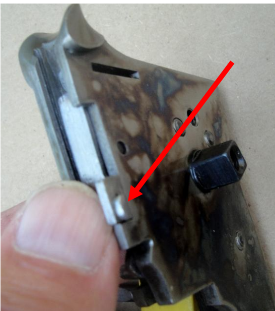
Install feeder arm-(arrow: nub fits hammer mortise)
