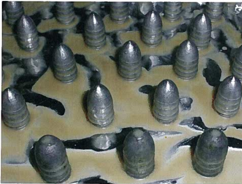
And the "baked bullets". Note that the closest three are .58 minie balls, rather than Sharps bullets. The lube flowed smoothly down and into the rings as well as smoothly coating the bullet surfaces.
