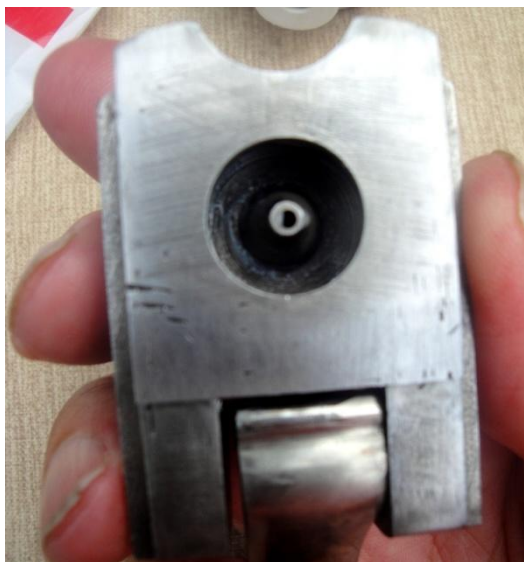
Cover O-ring with Lithium grease
