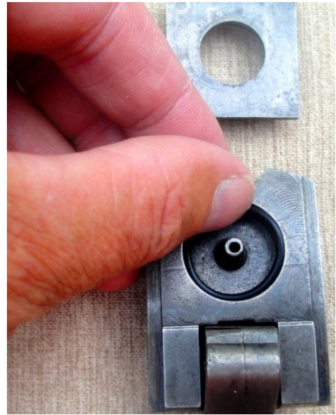
Step 2: Press O-ring into breechblock recess
