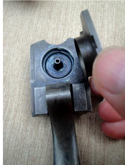
Return gas check into breechblock
