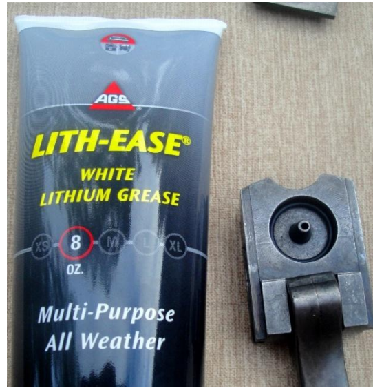
Lithium grease (used to protect O-ring)
