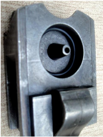
Side view of O-ring in block recess
