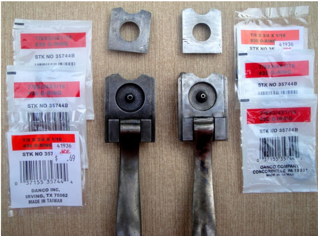
Garrett & Shiloh blocks, gas check plates (removed) and O-rings (Ace Hardware stock # 3744B 7/8 x 3/4 x 1/16)
