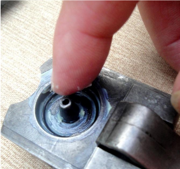
Cover O-ring with Lithium grease
